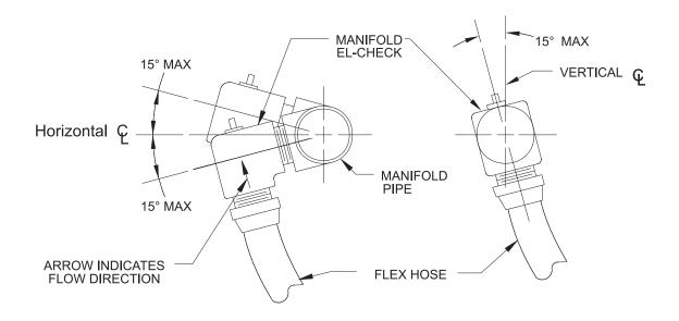
Note: Install El-Checks so that the arrow is in the direction, as indicated.
